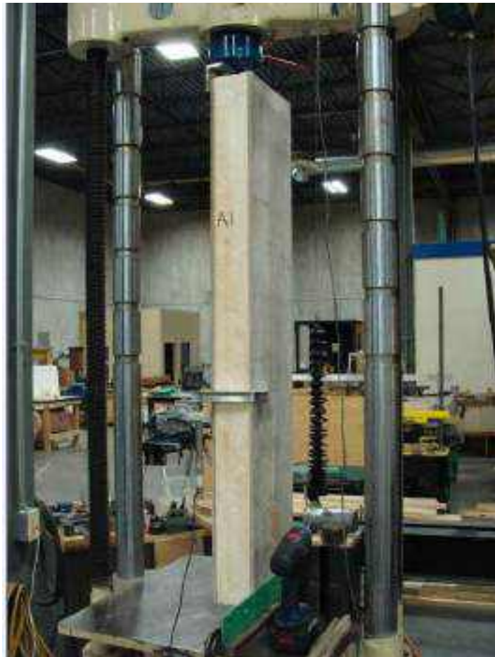
C273 Core Shear Properties Set-Up (“aged” specimen is shown)
