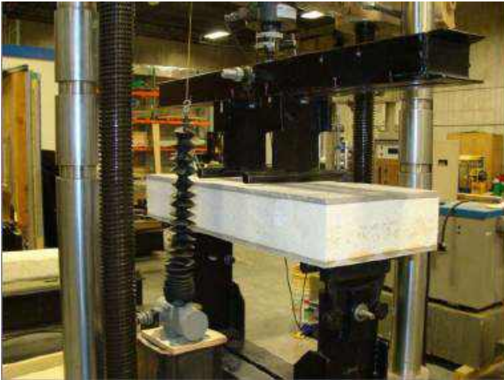
ASTM C393 Set-Up (“Control” is ready for test)
