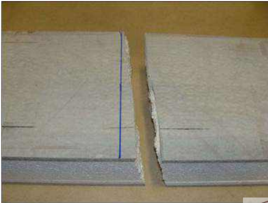
Typical failure for ASTM C393 “Control”
