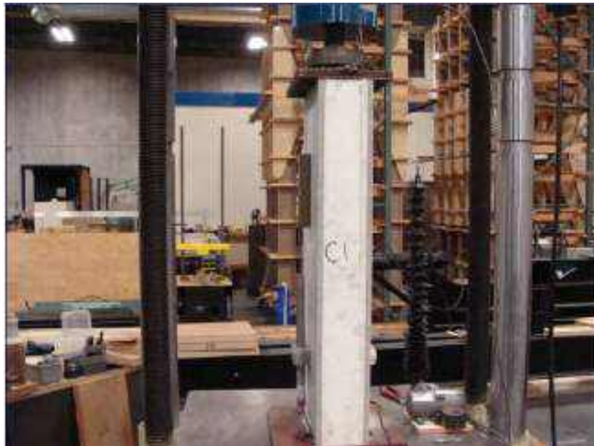
C364 Edgewise Compression Set-Up
